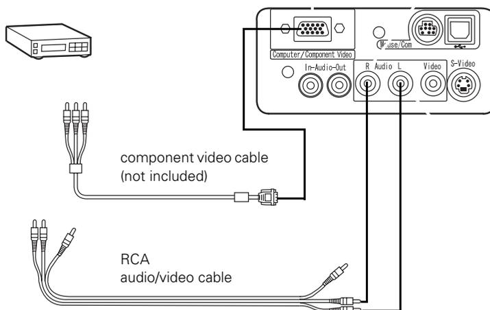
2. Connect the red and white plugs at the other end of the A/V cable to the corresponding audio output jacks on your video source.
