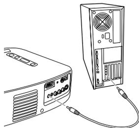
2. Connect the other end of the audio cable to the speaker or audio out port on the computer's sound card. If you don't need to make any other connections, you can plug in and turn on your equipment; see page 23 for instructions.
