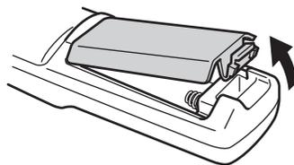
2. Insert the two AA batteries included with the projector as shown.
