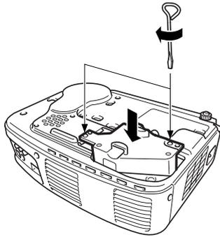
7. Insert the lamp cover as shown and press it back into place.
