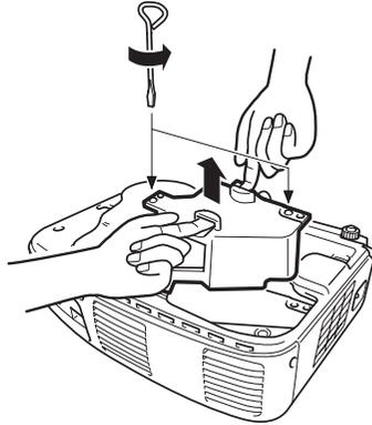
6. Position the new lamp correctly, then gently insert it into the projector. Press it into place and tighten the retaining screws.
