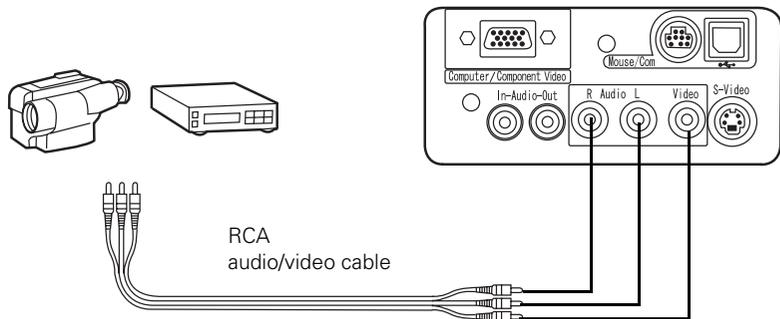
4. Connect the red and white plugs at the other end of the cable to the corresponding audio output jacks on your video source.
