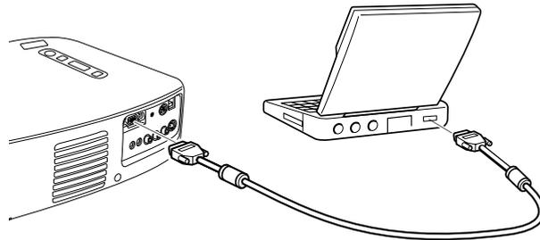
3. Tighten the screws on the connectors.
