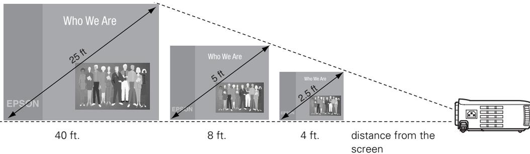
When projecting from a table, the ideal arrangement is to set the projector flat on its surface with the base of the lens at about the level of the bottom of the screen. This delivers the best-looking picture.
