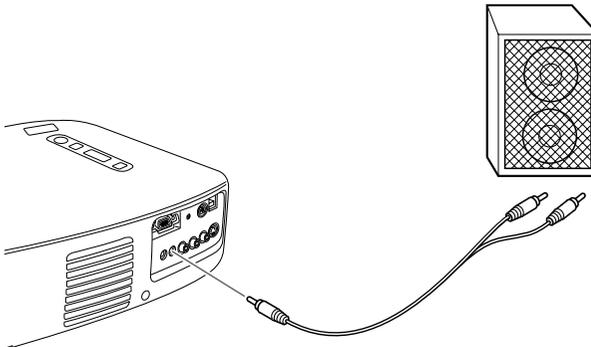
2. Connect the RCA plugs to the speaker or PA system. Insert the cable's red plug into the Audio R jack and the white plug into the Audio L jack.
