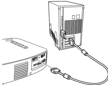
3. Connect the other end of the computer cable to the video (monitor) port on the Macintosh.
